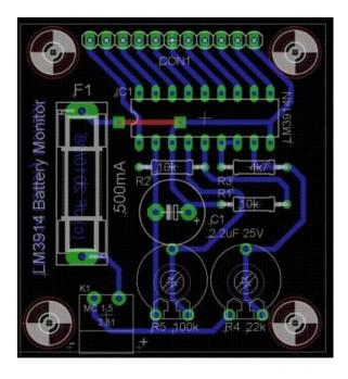
There's only one wire jumper that needs to be placed under IC1. All other components should be easy to place
