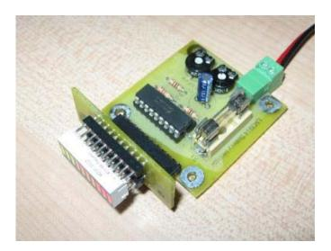
Voltages below 10V will turn off all leds and above 13.5V will maintain all leds lit.
